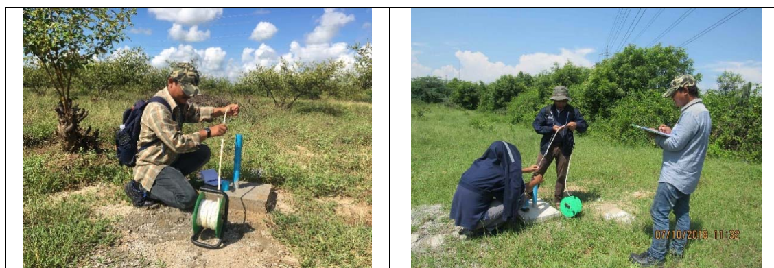
Figure 4.2-9 Scene of Ground Water Level Measurement
